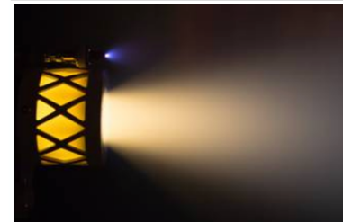
The Busek Company is developing Lunar IceCube's low-thrust electric propulsion system, the RF Ion BIT-3 thruster. Credits: Busek Company
