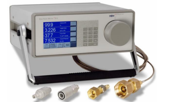
Optical chilled mirror dewpoint meter, MBW
