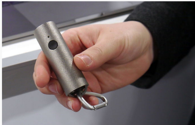
Figure 4. Atmotube is a portable air pollution monitor that detects a wide range of volatile organic compounds (VOCs) and harmful gases (e.g. Carbon Monoxide).
