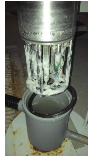
Multi sensor system to control process water of the paper industry left contaminated: right after cleaning with compressed air
