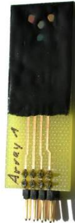
Si- substrate after PLD of the chalcogenide glass thin films and encapsulation
