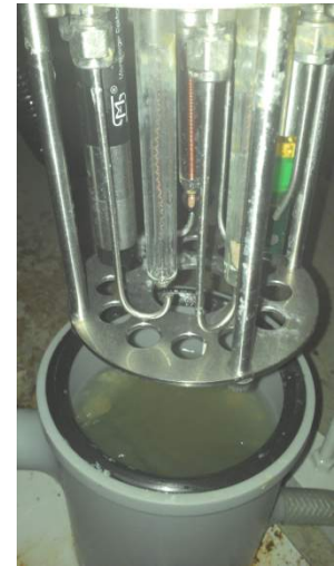
Multi sensor system to control process water of the paper industry left contaminated: right after cleaning with compressed air
