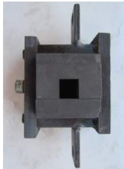
Two-piece graphite mold and of the glass pouring process
